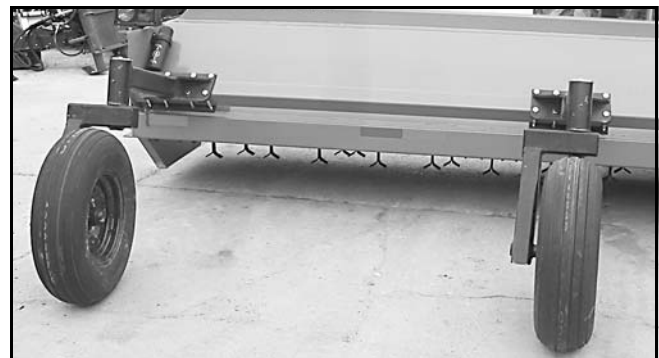
Figure 41. Wheel Assembly Installed
